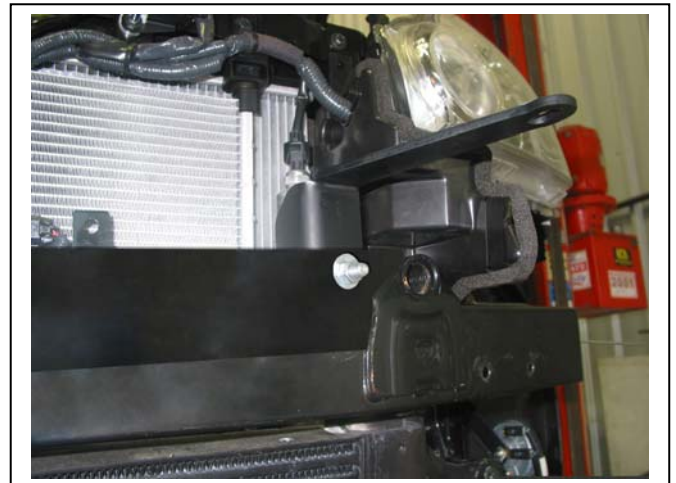
Figure 10 – ECB top support bracket fitted. Passenger's side shown.
